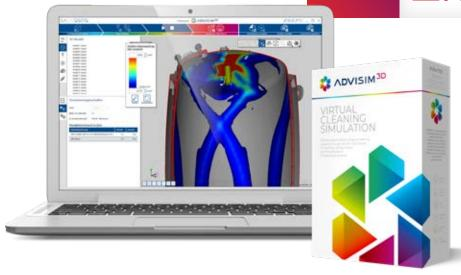
When designing and validating cleaning systems, the focus is always on the optimum nozzle configuration to remove contaminants from each individual point of the cleaning object in a resource-optimized manner. ADVISIM<sup>3D</sup> reliably visualizes spray shadows as well as the volume flow distribution and cleaning effect in its temporal progression.
